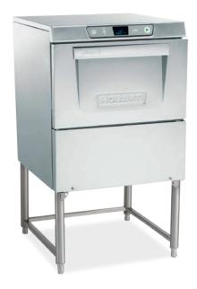
Hobart built the LXGeR to be cost efficient. Running entirely on a cold water line, the glasswasher incorporates an exclusive steam elimination and Energy Recovery system that captures steam from the wash cycle, then uses it for the next rinse cycle. This eliminates the need for hot water and results in a dramatic reduction of steam and up to \$485 in annual energy costs saved. And because it's a high-temperature glasswasher, the need to purchase expensive sanitizer is eliminated.
